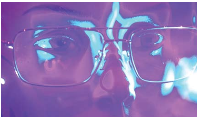
Figure 2 The letters 'UV' were seen reflected on the face of the mannequin by a standard lens while there was no such reflection from the Crizal UV lens
