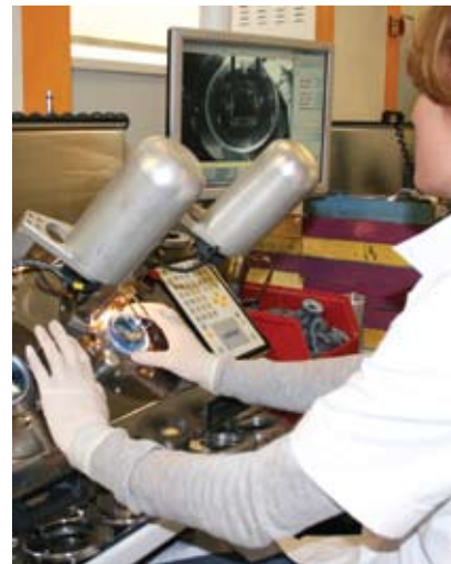
Traditional processes: lap tool polishing and finishing (top images) and lens blocking (left)
