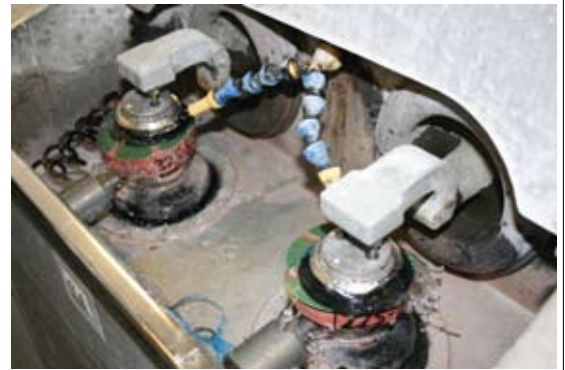
Traditional processes: lap tool polishing and finishing (top images) and lens blocking (left)
