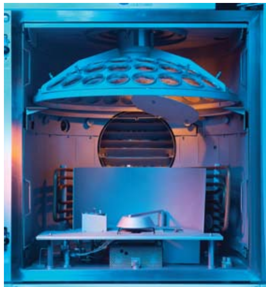
Vacuum chamber of the Satis Loh MC-380-X
