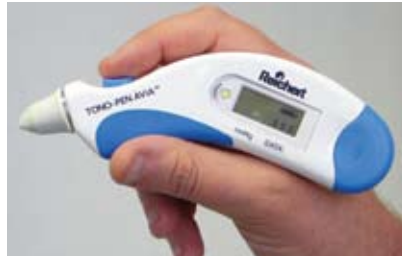
Figure 1 The Tono-Pen tonometer
