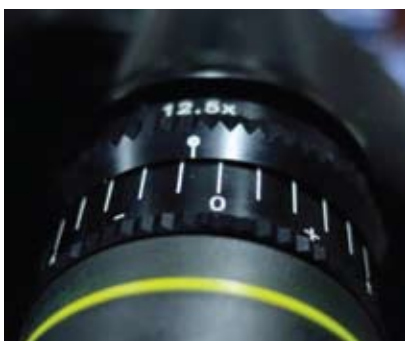
Figure 2 Using a correctly focused eyepiece with reticule can reduce focus errors
