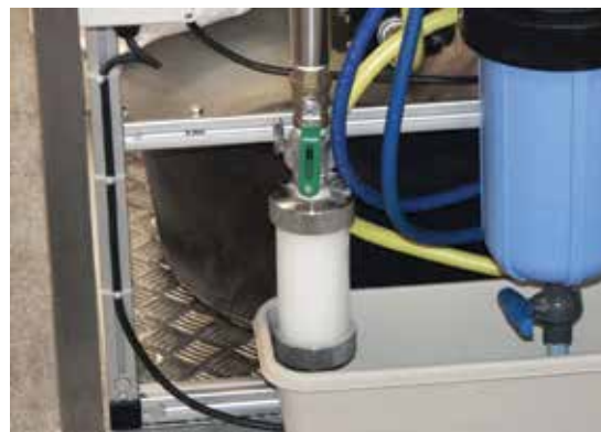
The Euro Aquasave isolates the plastic pieces, allowing clean water to be returned time and again
