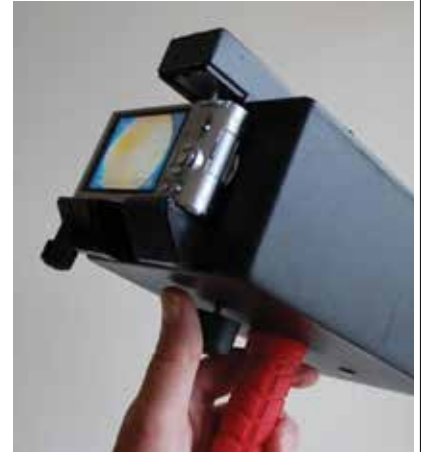
Figure 5 Thumb-operated shutter release
