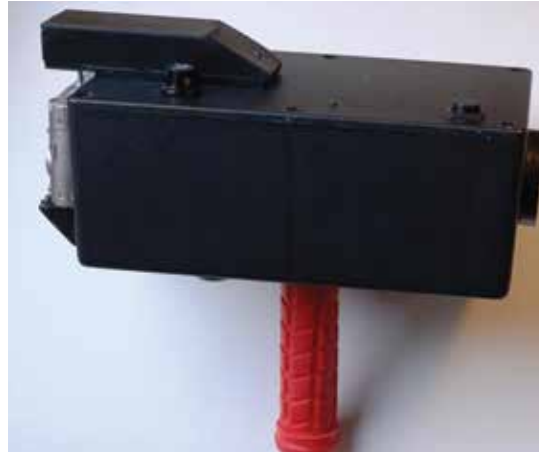
Figure 4 Hand grip for one-handed operation
