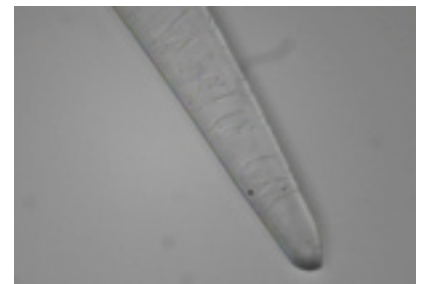
Figure 2 Edge profile for the Air Optix Individual lens, produced by the InnoLathe process
