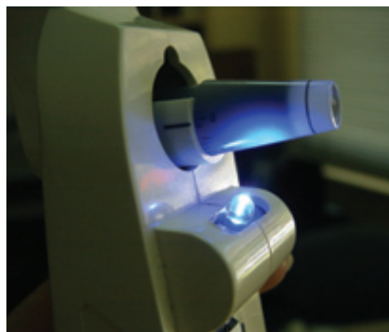
Figure 2 Perkins tonometer with LED illumination
