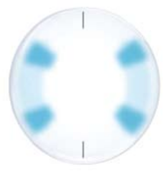
Figure 3 Accelerated Stabilisation Design of the Acuvue Oasys and Advance for Astigmatism lenses
