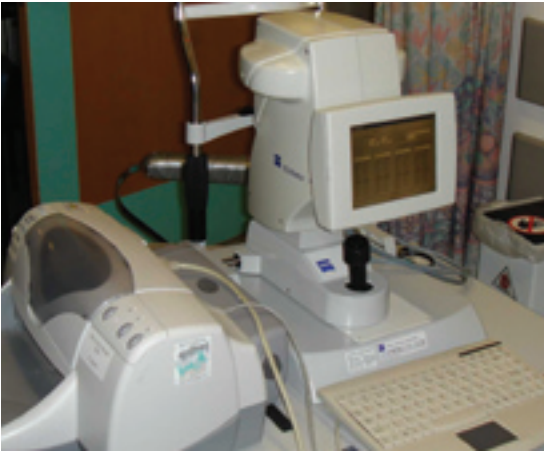
Figure 4 IOL Master (Zeiss) used in biometry measure- ments prior to cataract surgery
