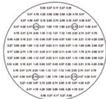
Figure 7 Free-form description of a hyperboloidal surface of power -5.50D and p-value -3.6, worked on a material of refractive index 1.60. The z-values listed are the sags of the surface for the x,y coordinates which are given in 5mm intervals from the centre out to 35mm. The four circled values represent the coordinates (±15, ±20, 2.74)
