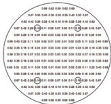
Figure 8 Aberration filter expressed in digital form. The four circled values represent the coordinates (±15, ±20, 0.16) where the value, 0.16, represents the adjustment to the z-coordinate (aberration filter) applied to this point
