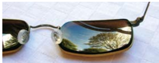
Figure 4 Rear surface of uncoated tinted lens acts as excellent concave mirror
