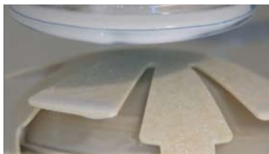
Figure 3 The CNC controlled flexible lap tool
