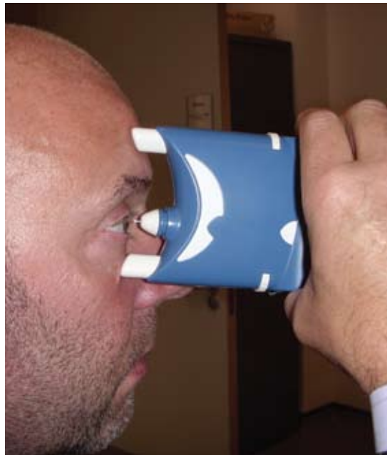
Figure 2 Two guides above and below the orbit help position the instrument correctly
