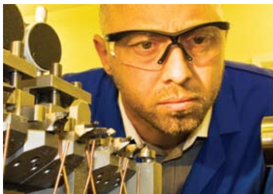
Figure 1 Production director Garth Barnard pictured with the Optoform 40 lathe used to make Nissel K2 Rigid lenses
