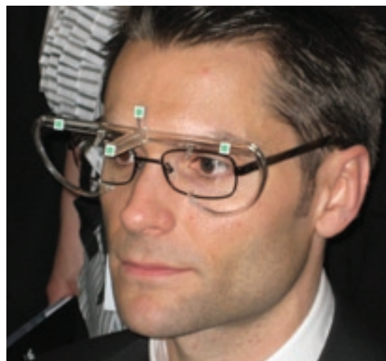
Figure 3 The frame with four sensors for measurement
