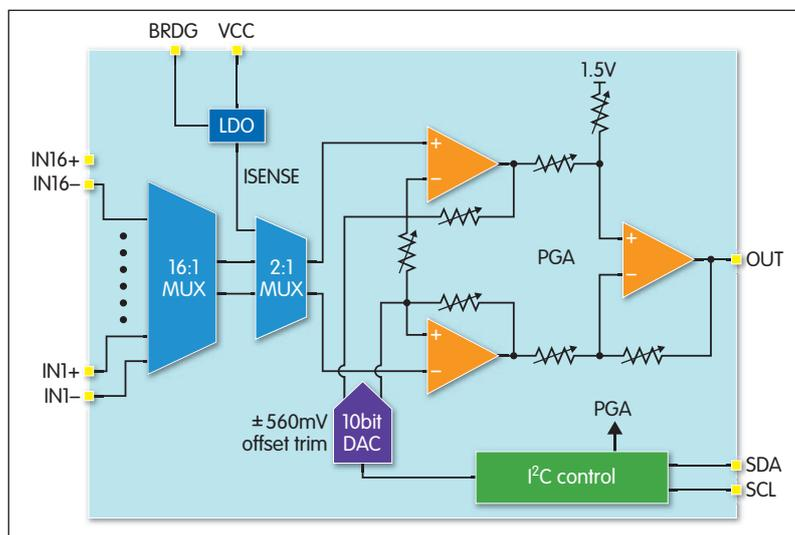
Fig 1: Block diagram of Exar's XR10910 analogue front end
