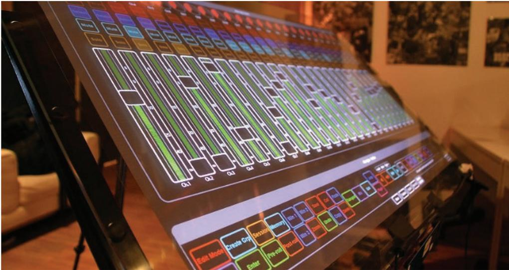
for a 16:9 aspect ratio and provides a uniform response to touches across the whole area. This optimisation, CDS contends, results in a more accurate and precise touch detection.
