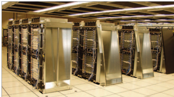
The Blue Brain project at EPF Lausanne is using an 8192 processor version of IBM’s Blue Gene supercomputer in order to model the brain’s functionality in real time.
