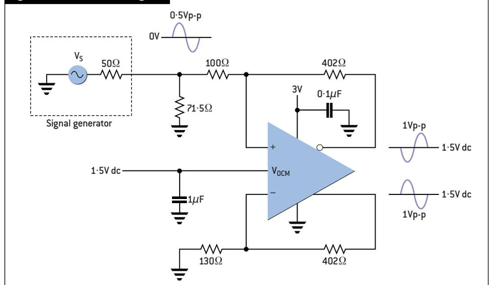
can trade off stability at lower gains for better performance at higher frequencies. The LTC6404 is available in three versions: unity gain stable; and gains of 2 and 4. Operating from a single 2.7 to 5.25V supply, the part has rail to rail outputs, allowing output swing to be maximised.
