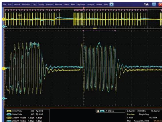
**Figure 3:** Using Advanced Search & Mark to identify all write bursts.
