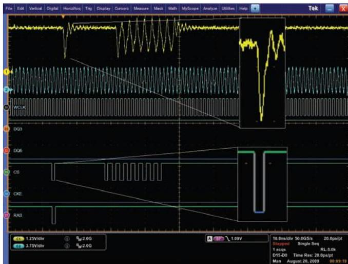
**Figure 9:** iCapture showing Chip Select line with analogue and digital views.
