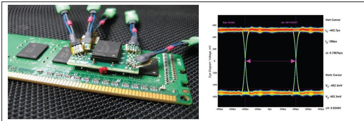
**Figure 2:** Component Interposer with solder tips; eye diagram of probed signal.
