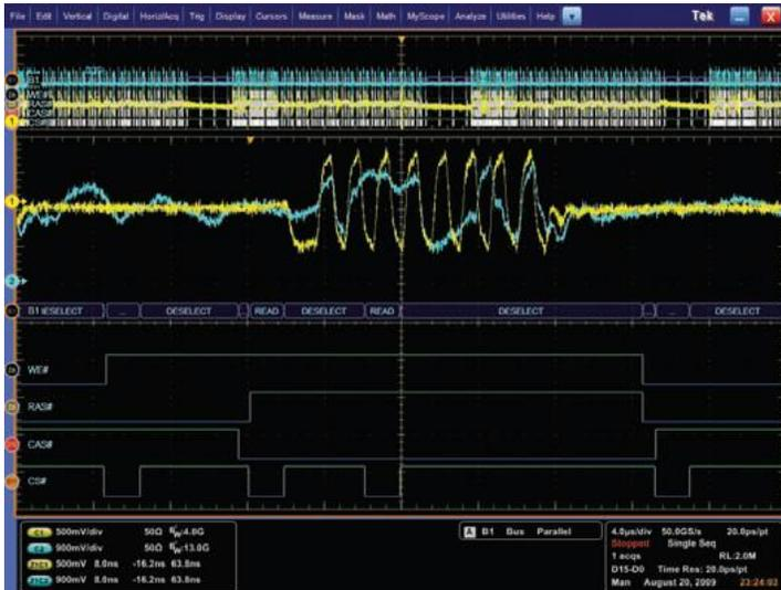
**Figure 5:** DDR3 Command Bus decoding on MSO70000.
