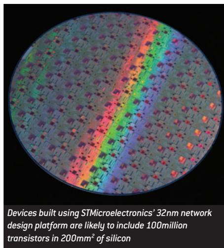
Devices built using STMicroelectronics' 32nm network design platform are likely to include 100million transistors in 200mm<sup>2</sup> of silicon
