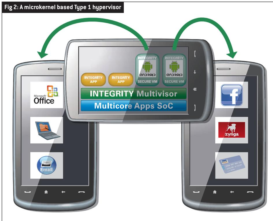
Fig 2: A microkernel based Type 1 hypervisor
