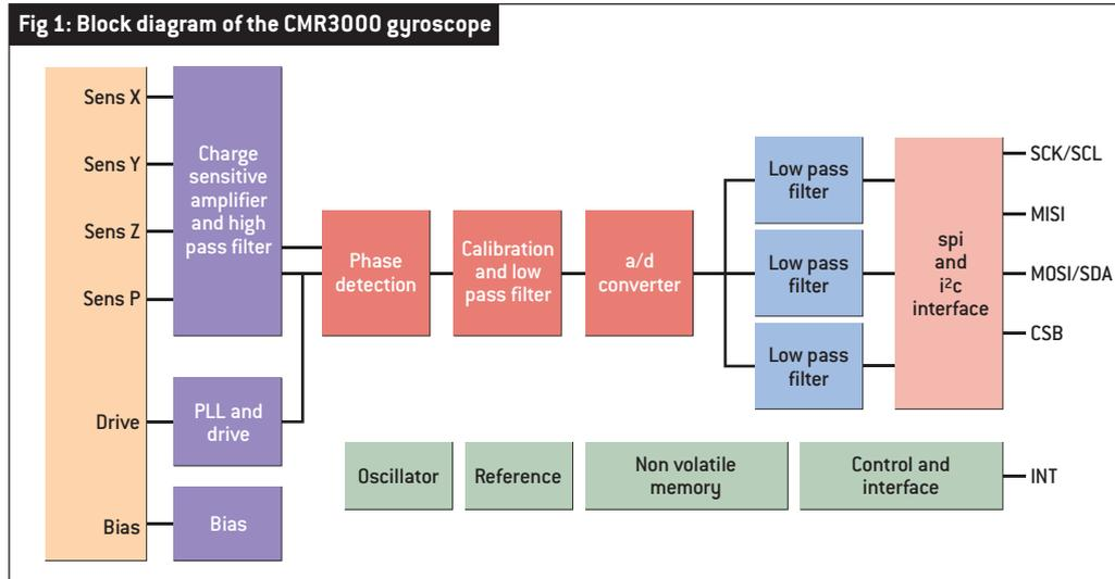
signal conditioning ASIC. An internal oscillator, reference and non-volatile memory allows the sensor to operate autonomously within a system.
