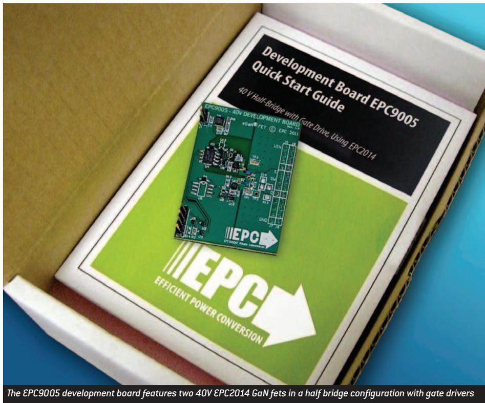
The EPC9005 development board features two 40V EPC2014 GaN fets in a half bridge configuration with gate drivers
