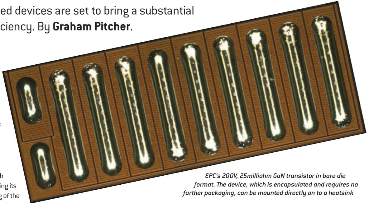
*EPC's 200V, 25milliohm GaN transistor in bare die format. The device, which is encapsulated and requires no further packaging, can be mounted directly on to a heatsink*
