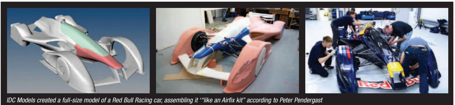
*IDC Models created a full-size model of a Red Bull Racing car, assembling it "like an Airfix kit" according to Peter Pendergast*
