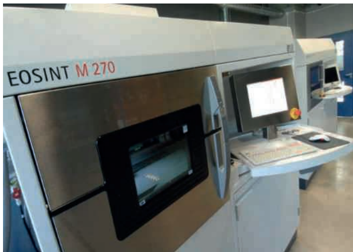
One of the sintering machines in action at CRDM and [right] direct metal laser sintering of maraging steel powder
