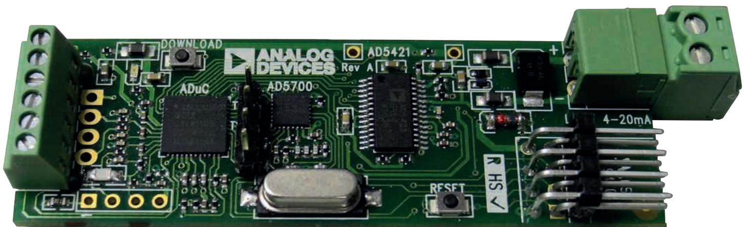
Fig 1: A smart transmitter signal chain
