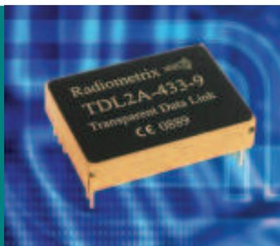
TDL2A, a multichannel uhf transceiver capable of emitting 10mW of transmit power. Operating in the European unlicensed 433MHz ISM band, it can support data rates of up to 9600bit/s and has five non overlapping channels at its disposal.
