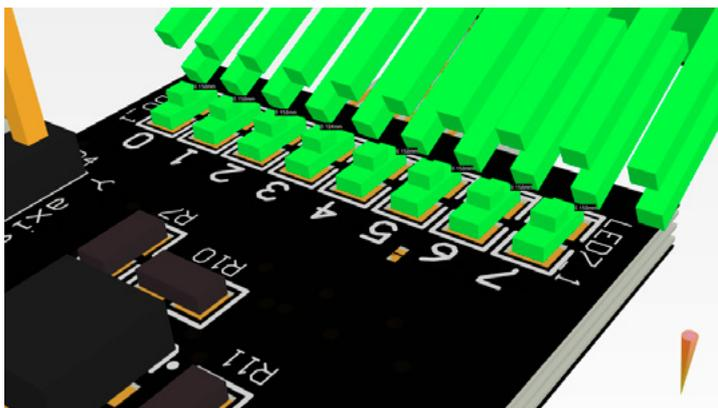
*Fig. 5: Simulated bending of a flex circuit reveals a clearance violation between a flex-mounted pin-header and SMDs on the main rigid board. The violating components are highlighted green. <sup>7</sup>*
