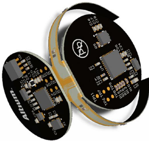
*Fig. 4: An example rigid-flex PCB design in Altium Designer's 3D mode, showing intended bends in the flex-circuit areas. <sup>7</sup>*
