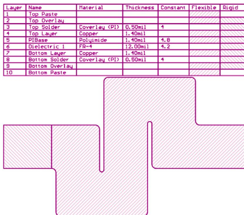
Fig. 2: Fill patterns in the “Flexible” and “Rigid” columns in the table identify the rigid and flexible areas of the board. <sup>3</sup>
