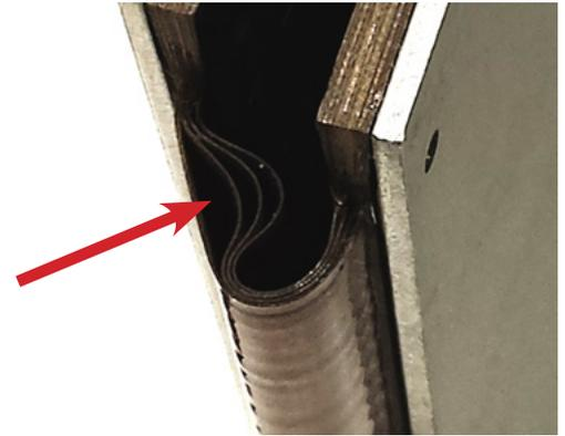
*Fig. 3: In this commercially produced design, the designers obviously did not apply “bookbinder construction”, resulting in additional stress on the separated layers (red arrow).<sup>7</sup>*
