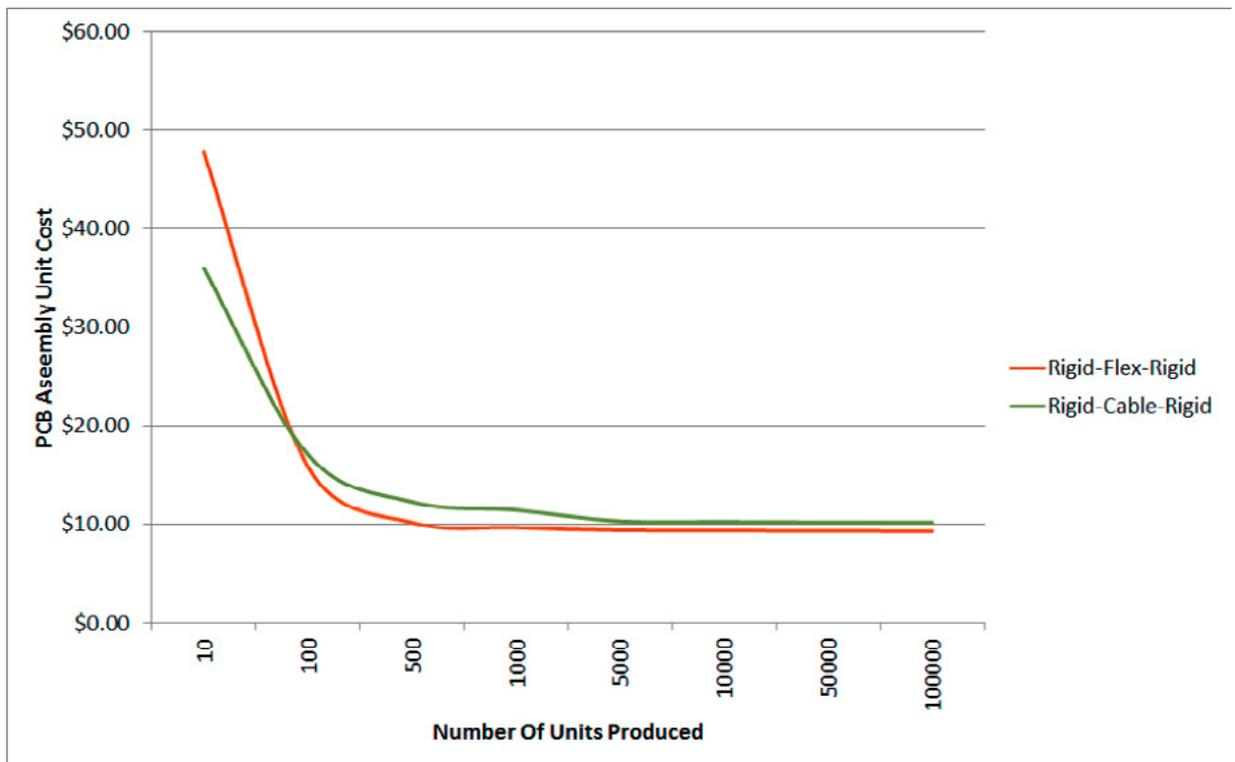
Figure 1: Quote-generated cost comparison of Rigid-Flex design versus Rigid-Cable-Rigid PCB assembly.
