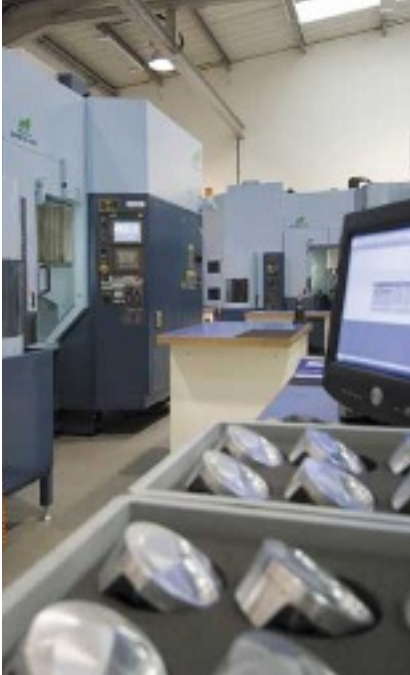
The two Matsuura machines almost fill the available space. In adjacent temperature-controlled room, the Takisawa CNC lathe comfortably achieves 0.003 mm
