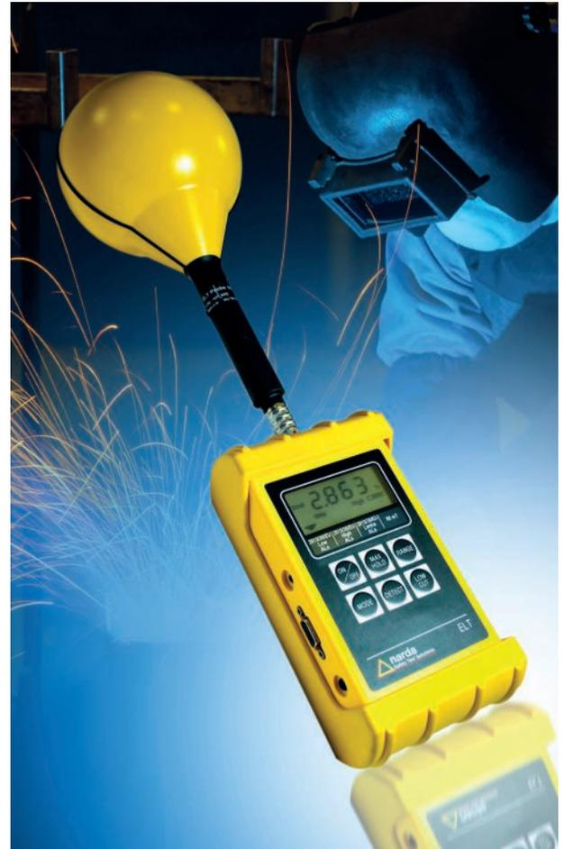
Magnetic field strength meters provide an easy means of proving compliance with the CEMFAW Regulations
