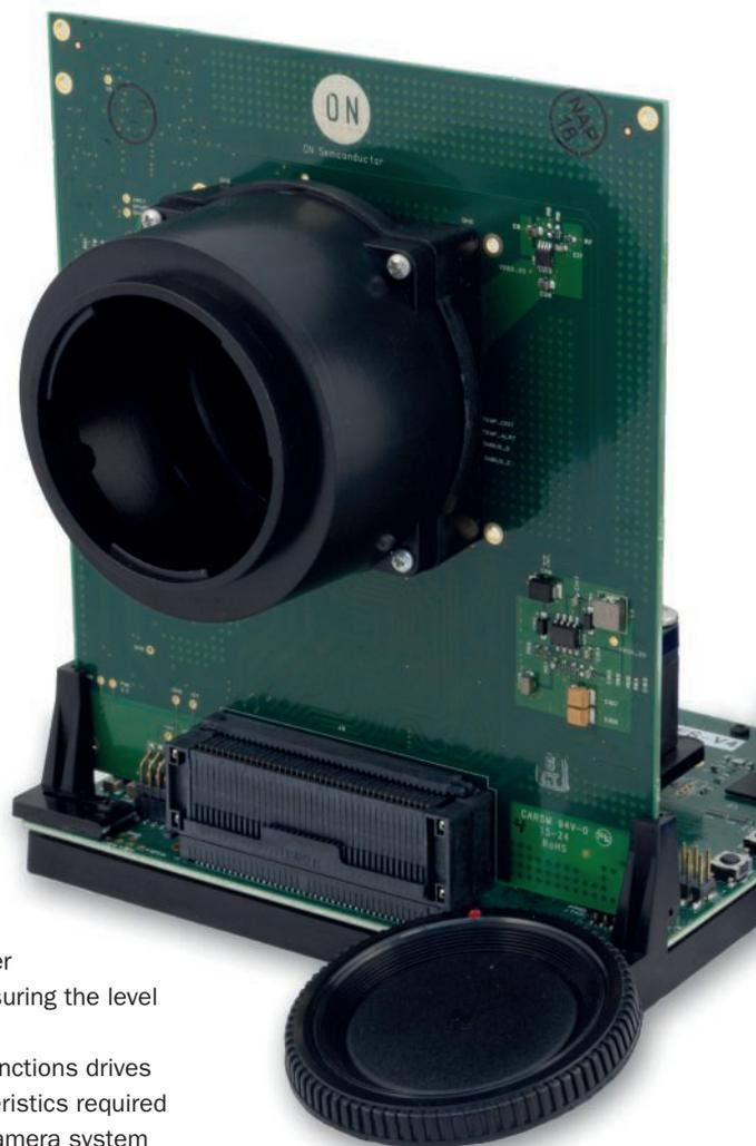
that enables the capture of moving objects without the introduction of motion artefacts. In-pixel correlated double sampling provides low readout noise, while on-chip fixed pattern noise correction helps preserve image quality. Combined with a 10bit A/D converter and a dynamic range of 60dB, these features allow machine vision systems to leverage the intrinsic advantages of a CMOS platform in their operation.
