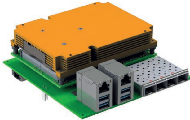
Figure 3: The Mini-STX form factor is about twice the size of the eNUC form factor but 29% smaller than the Mini-ITX form factor.
