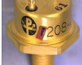
Coarse Leak “Failure site”
