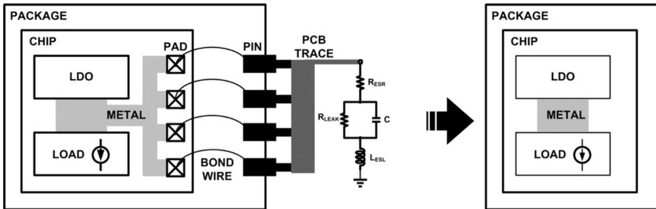
Figure 2. Off-Chip Capacitor LDO versus Capless LDO
